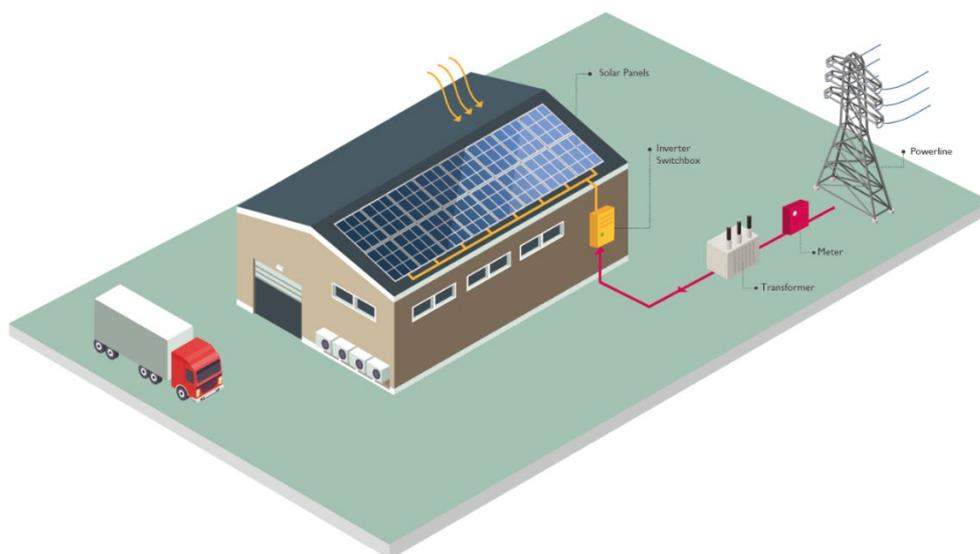
**Figure 7 Business customer with Behind-the-meter solar PV installation**
