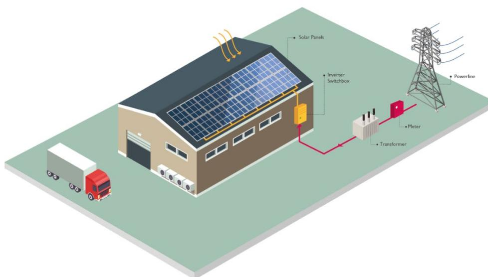
**Figure 5 Business customer with Behind-the-meter solar PV installation**
