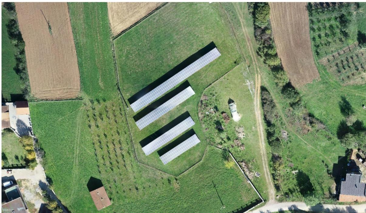
**Figure 17 Gjurgjevik, Klinë, 102 kW Solar PV based on Feed-in Tariffs**
