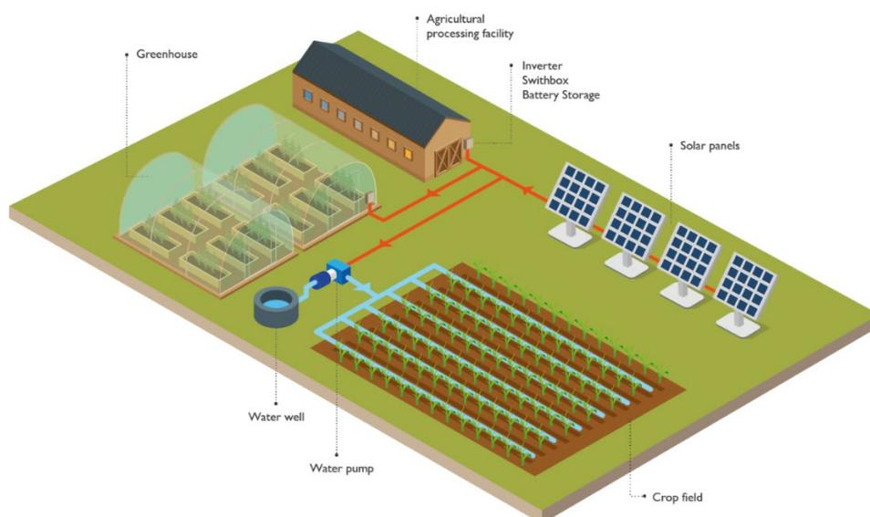
**Figure 7 Off-grid solar PV generator in agriculture**
