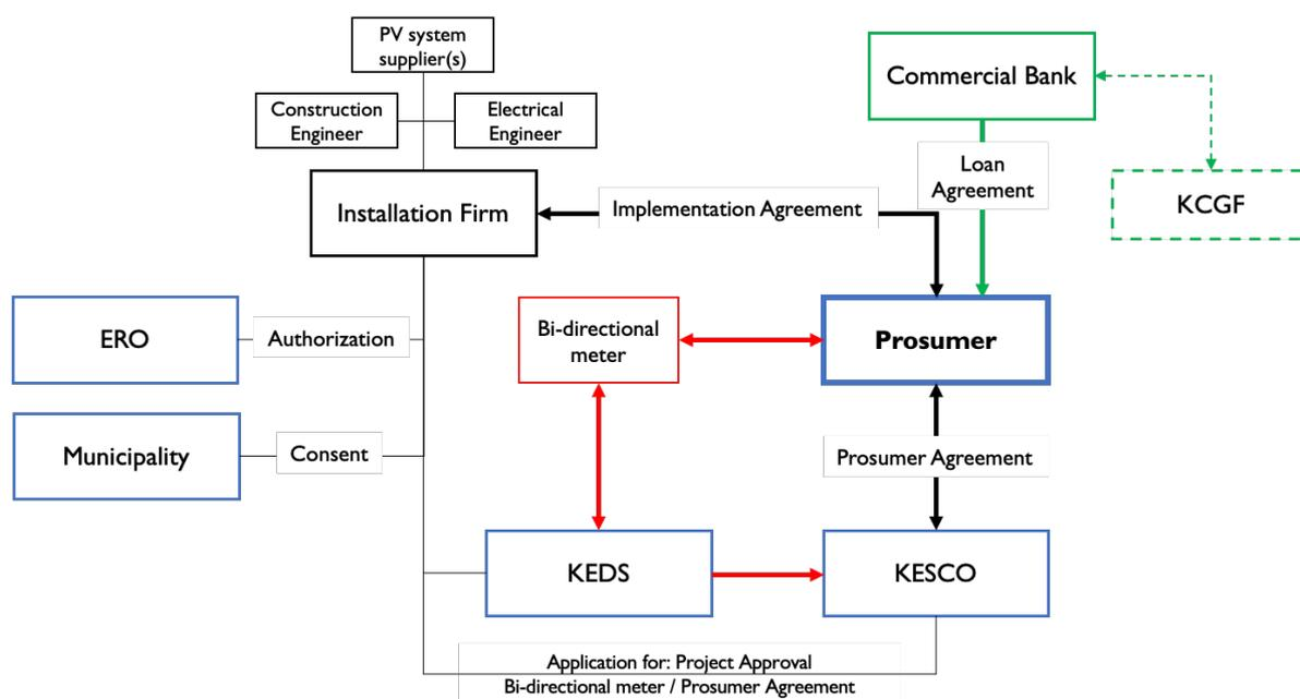
**Figure 6: Schematic of a Typical Prosumer Installation**
