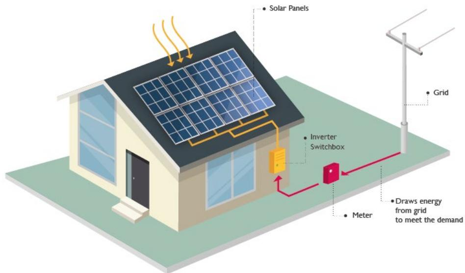
**Figure 6 Behind-the-meter generator**
